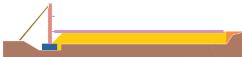
Fig. 1.7 : Connect and tighten Reinforcement (source : MSE Wall Inspector's Handbook, Paul D. Passe 2000)
