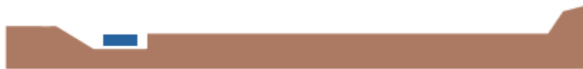
Fig. 1.3 : Place concrete leveling pad (source : MSE Wall Inspector's Handbook, Paul D. Passe 2000 )
