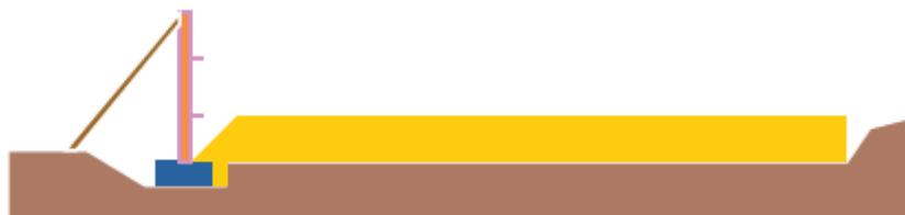
Fig. 1.6 : Fill in 6" lifts to reinforcement (source : MSE Wall Inspector's Handbook, Paul D. Passe 2000)
