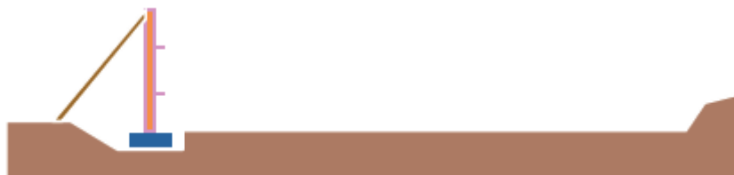
Fig. 1.4 : Install and brace 1 st row of pannels (source : MSE Wall Inspector's Handbook, Paul D. Passe 2000 )
