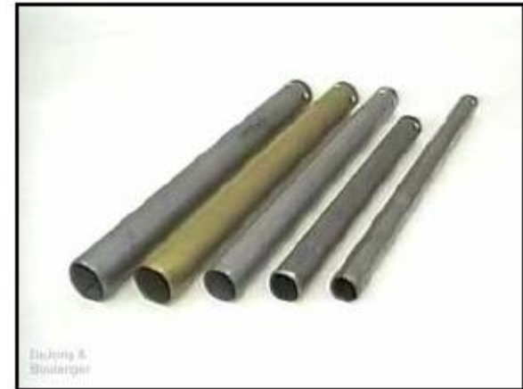
Figure 3-11: Selected Sizes and Types of Thin-Walled Shelby Tubes.
