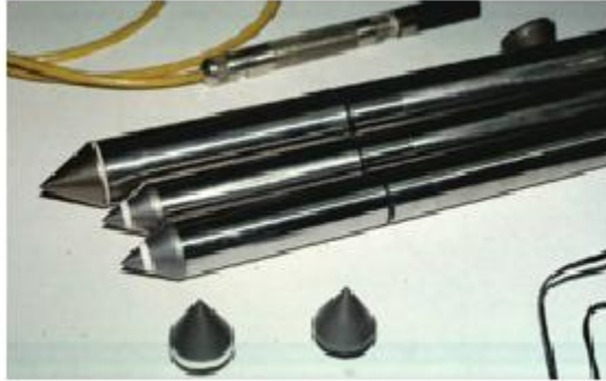
Figure 5-5. Various Cone Penetrometers Including Electric Friction and Piezocone Types.
