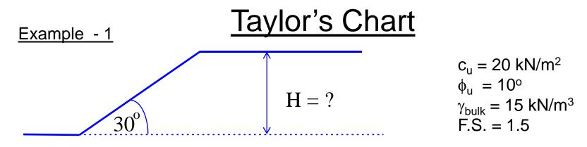
Since the factor of safety is given, then the problem indicates a design of a new slope
