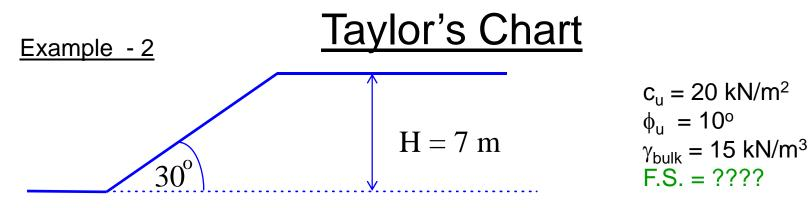
Since the factor of safety is not given, then the problem indicates an existing slope which we need to analyze it for its stability.
