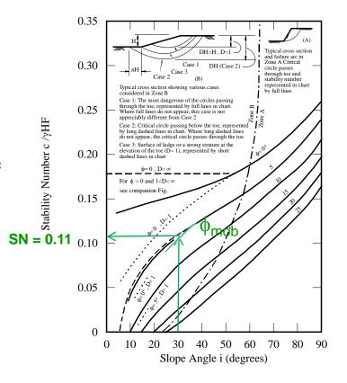
Since we complied three different trials, we are ready to find the right factor of safety by using the 45° line method
