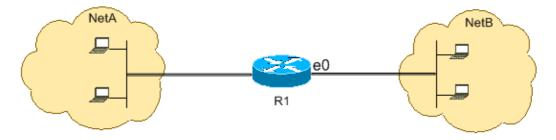
The following configuration, permits only echo-reply (ping response) packets to come in on interface Ethernet 0 from NetB toward NetA. However, the configuration blocks all echo-request ICMP packets when
