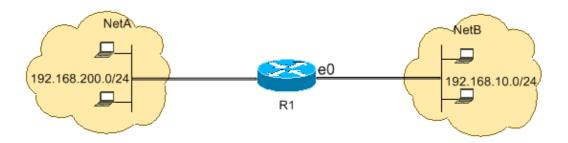
The following configuration allows the IP packets whose IP header has source network number of 192.168.10.0/24 and a destination network number of 192.168.200.0/24 access to NetA. Again, there is the implicit deny all clause at the end of the ACL which denies all other traffic passage through Ethernet 0 inbound on R1.
