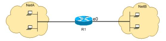
Telnet uses TCP, Port 23. The following configuration shows that all TCP traffic destined to NetA for Port 23 is blocked, and all other IP traffic is permitted.
