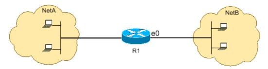
The following configuration permits TCP traffic with destination port values matching WWW (port 80), Telnet (port 23), SMTP (port 25), POP3 (port 110), or FTP (port 21). Notice an implicit deny all clause at the end of an ACL denies all other traffic, which does not match the permit clauses.
