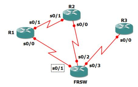
Refer to FRSW.txt for the configuration of FRSW (Frame Relay Switch). DLCI 102 is connected to DLCI 201; DLCI 103 is connected to DLCI301; and DLCI 203 is connected to DLCI 302.
