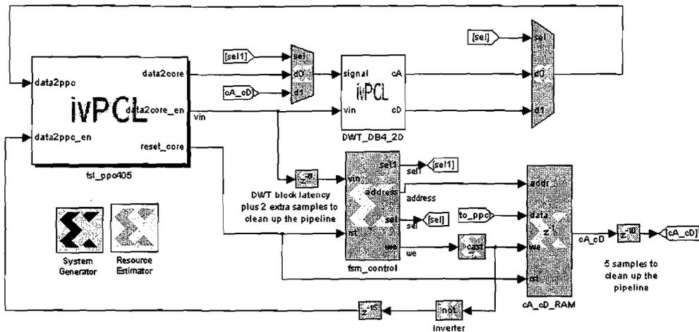
Figure 7. Sysgen's 2D DWT model.
