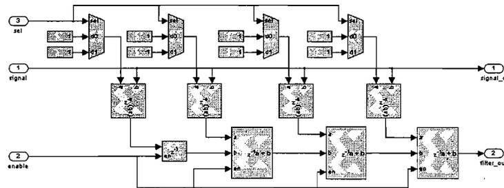
Figure 12. Structure of decimator/filter using embedded multipliers blocks and time multiplexion to reduce resource consumption.
