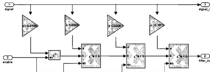
Figure 13. Structure of decimator/filter using constant multipliers blocks. In this case, the multipliers can be implemented using Distributed RAM (DRAM) or Block RAM (BRAM).
