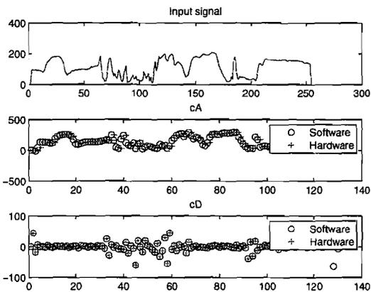
Figure 8. Hardware co-simulation results for a 1D single stage DWT.
