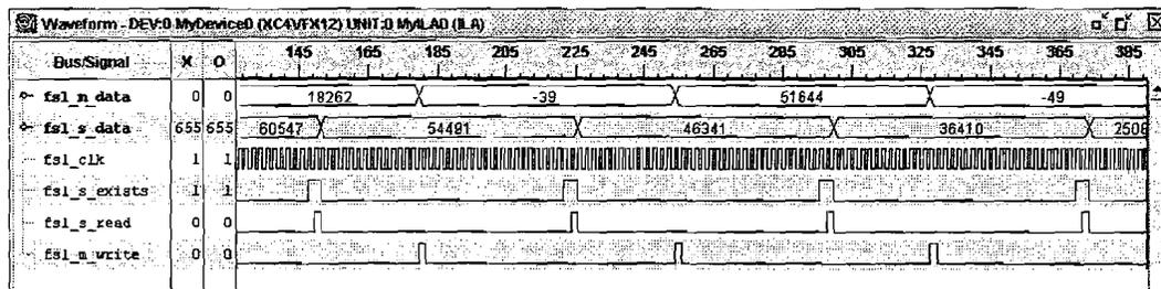
Figure 16. Bus interface validation using Chipscope 8.2.
