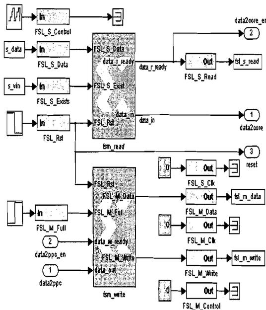
Figure 3. Internals of the block in Fig. 2. The block is basically built upon finite state machines to control the signals for reading and writing to and from the FSL bus.
