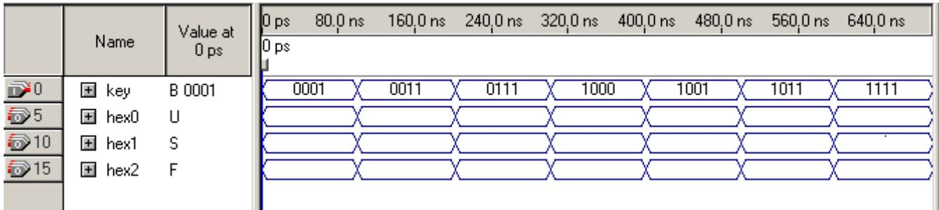
6. Now go back to the **Simulator Tool** window. Run the **Generate Functional Simulation Netlist**, select **Overwrite simulation input file with simulation results** and deselect **Automatically add pins to simulation output waveforms**. Finally hit the **Start** button to run the simulation. Answer with **Yes** to overwrite the current simulation results.
