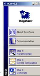
6. Now go back to the NCO v9.1 ToolBench window. Skip **Step 2** and click on **Step 3: Generate.** Several output files are generated including a `NCO.html` file that gives an overview over the generated files. Study the short description given in the html file. Finally click **EXIT** to exit the ToolBench.
