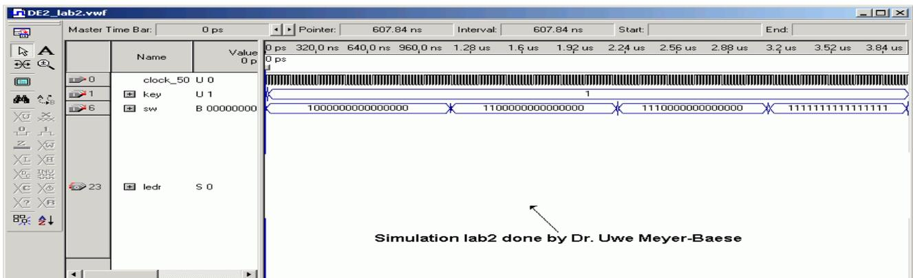
Start the functional simulation after generating the netlist and then change the *ledr* waveform to **Analog** with **Style Step** and **height 10**. Print the completed waveform including your e-signature.
