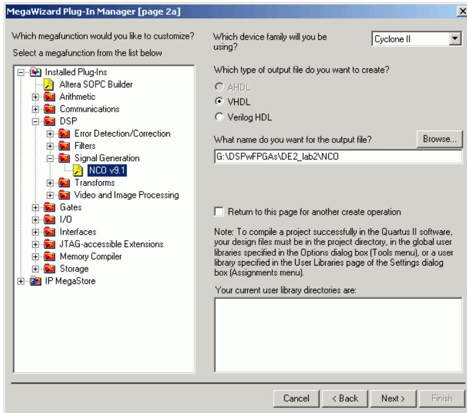
3. Then click **Next >** and the IP ToolBench will load. You may want to read the **About** and the **Documentation** first. Next click on **Step1: Parameterize** and make the following setting in the first **Parameters** windows of the core.
