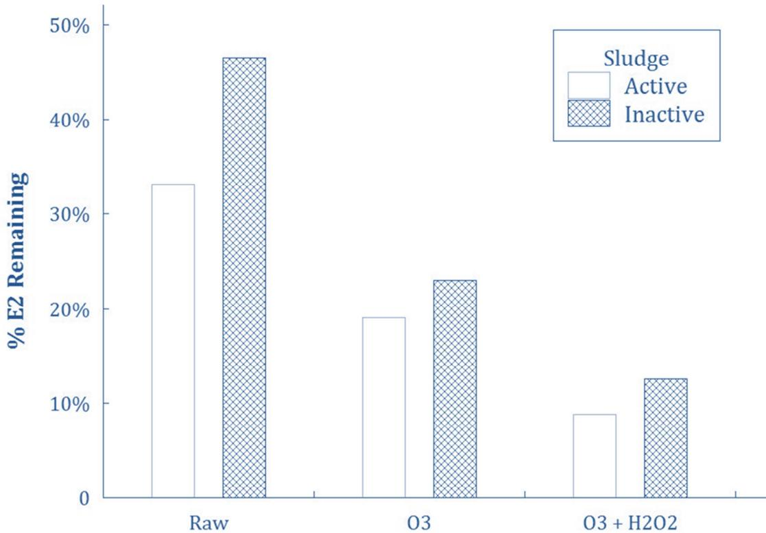
Figure 1 – Degradation of E2 in Leon County leachate under anaerobic conditions (batch) after pre-treatment with ozone or ‘peroxone’ (H<sub>2</sub>O<sub>2</sub> + O<sub>3</sub>). Incubation: 24 hrs.
