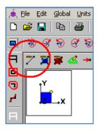
We will see the **member properties** dialog. Select Concrete from Member Material Type. In the release codes select Fully Fixed at Both Ends. Pinned structure would be related to truss structure. Our frame has fixed joints. Click Apply to draw members. To assign the shape directly click on button encircled in the figure below.
