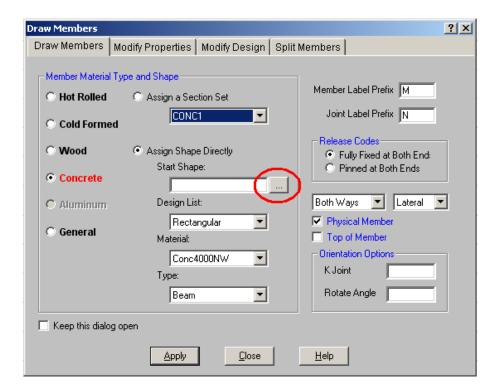
Define size of the Beam element cross section as your initial design assumptions show. In our case outer dimensions of all beams are 36in (depth) and 20in (width).
