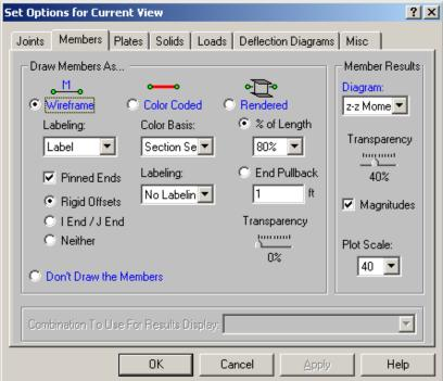
From Members card choose z-z Moments in Diagram and check Magnitudes. By applying that we should get envelopes of bending moment envelope for all members like in the figure below.
