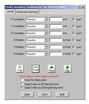
Hit Apply. The mouse cursor now looks like this  $\stackrel{\triangle}{\triangle}$ , which indicates that you are ready to apply the boundary condition to any joint that you click on. We want to apply the boundary condition to the base of both columns at joints N17 to N20. Right click to end the command.
