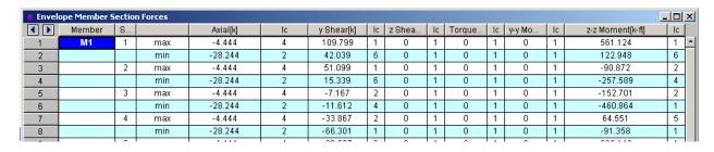
Knowing the load combination # that caused extreme value of force we can perform quickly once again analysis for that particular combination. For member 1 (beam in bending) we are interested in biggest absolute values of shear and moment. We will be considering:
