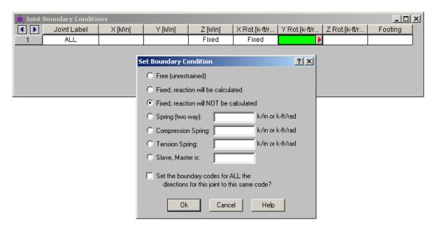
Enter all values, hit OK and end the Joint Boundary Conditions window. Note: If a joint is explicitly listed with boundary conditions, those boundary conditions override the "ALL" conditions for all 6 directions. The "ALL" specified boundary codes apply only to those joints NOT otherwise listed on the **Boundary Conditions Spreadsheet**. This is why joints 1 and 2 in the figure above also have the Fixed code in the Z translation, 2x Rotation and 2y Rotation fields.
