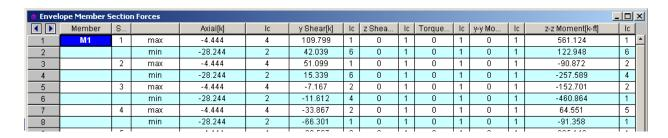
For member M1 we see results for 5 different sections. Number of sections through the element is defined in Global Parameters in solution card. Sometimes default value of 5 is not enough. Increase slightly that value for your project (let's say 7 or 9) and repeat the solution. For each section we get min and max value of axial force, shear forces and moments. Also we get in columns Ic the load combination that caused extreme value of internal force.
