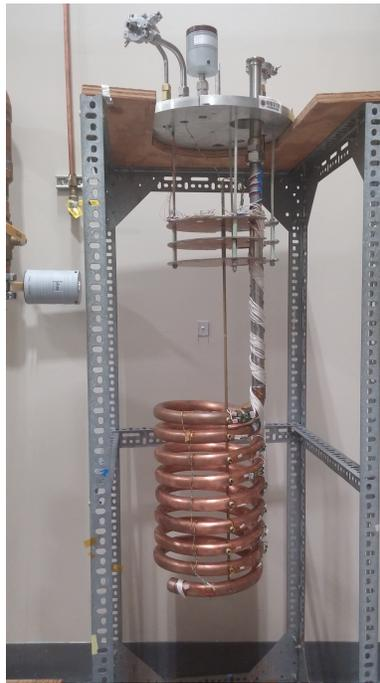
Figure 2.2: Initial helical tube setup after fabrication.
