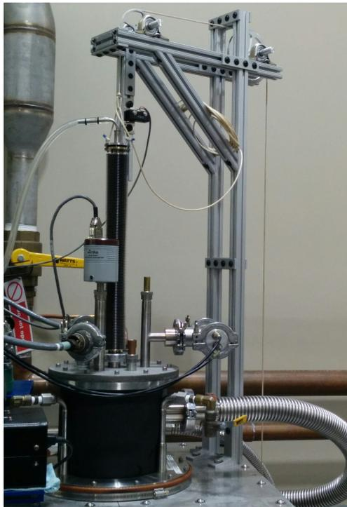
Figure 2.9: Photograph of the top of the cryostat, showing the bellows and a portion of the pulling cable system.
