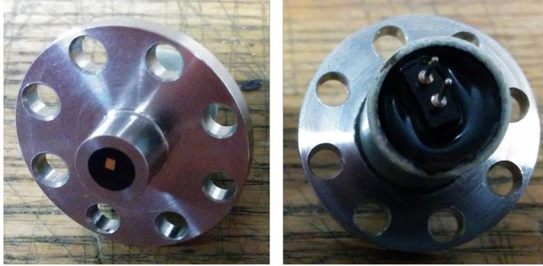
Figure 2.6: Photographs of the (left) sensing side and (right) connector side of the temperature sensor assembly.
