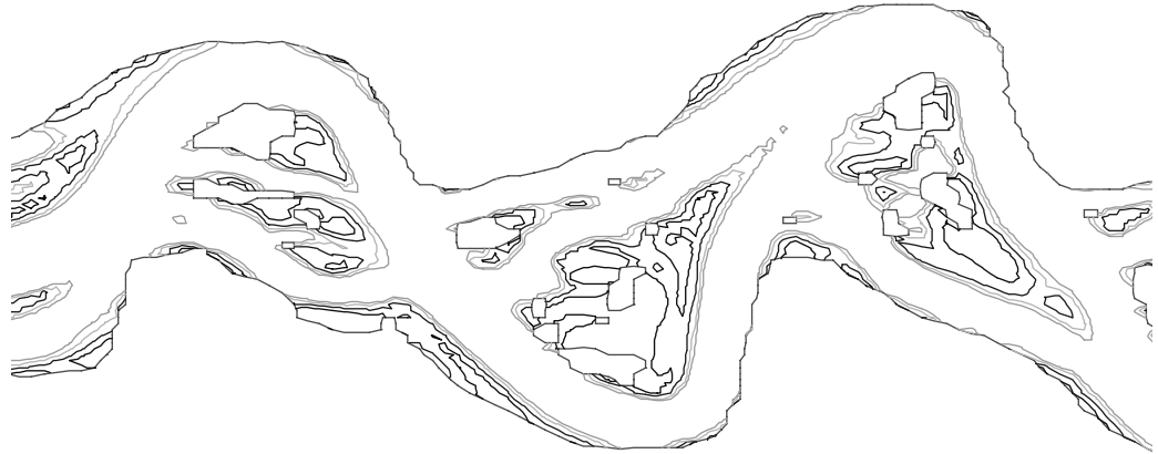
Figure 9.8.9 Plan view of depth-average water velocities in a meandering river, where cutoffs have started to make a braided plan form.
