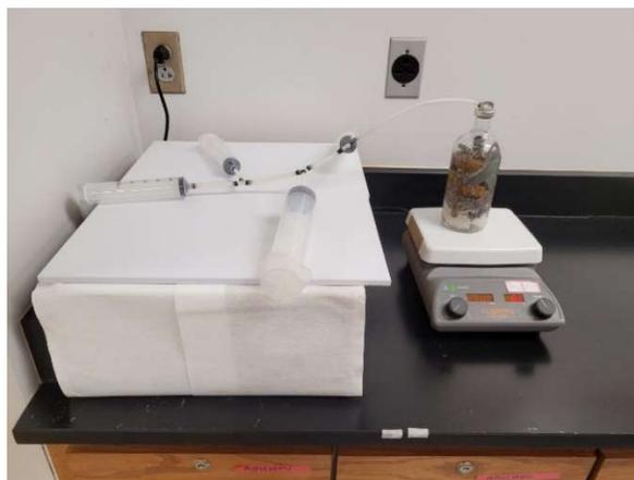
**Figure 2.4:** A lab-scale landfill for evaluating the fate of PFAS in solid waste
