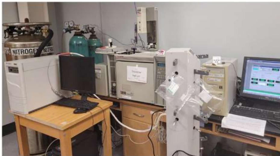
**Figure 2.1:** A gas chromatography – mass spectrometry system coupled with a 7100 pre-concentrator for measurement of volatile PFAS
