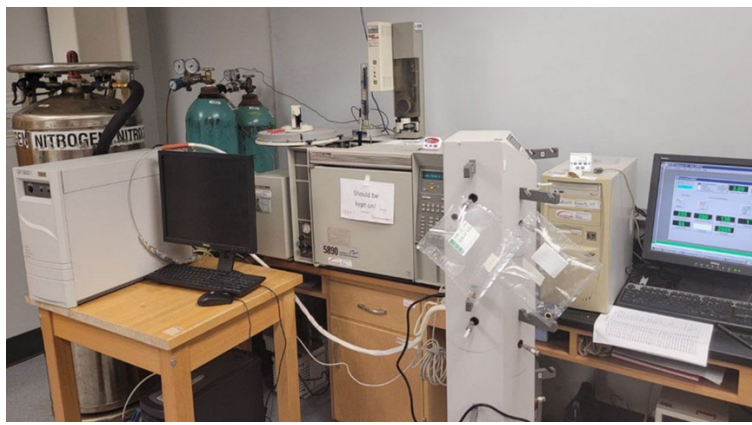
Figure 1. The system in the lab for gas-phase PFAS identification and quantification
